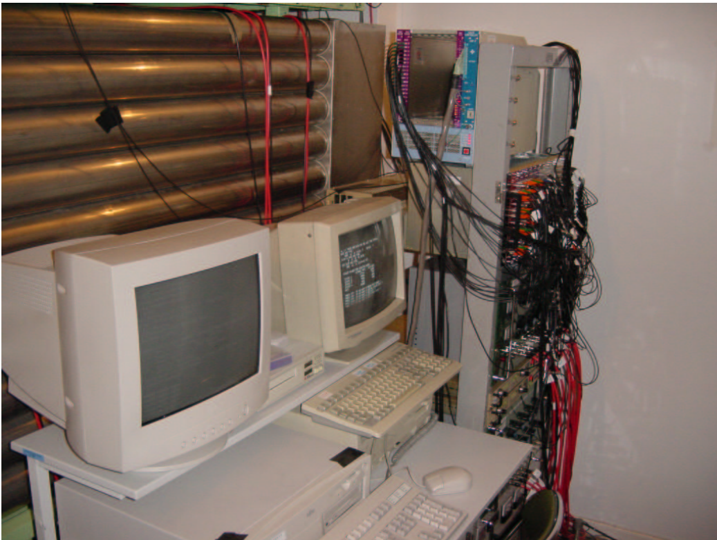
Figure 1.4: The SONTEL laboratory container at Gornergrat with the two data-taking computers (left), the electronics rack (right), and the proportional counter tubes (back).
